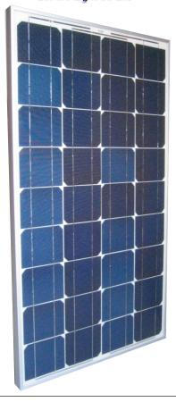
The **new** photovoltaic modules **IS100P** - **100Wp** and **IS110P** - **110Wp** are composed of **36** high efficiency monocristalline solar cells **156x125mm** produced with the most innovative technologies of isotropic texturization and antireflecting coating.
