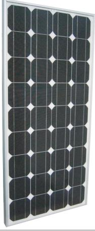
The new photovoltaic modules IS75P - 75Wp and IS90P - 90Wp are composed of 36 high efficiency monocrystalline solar cells 125x125mm produced with the most innovative technologies of isotropic texturization and antireflecting coating.
