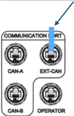
CAN communication from HV BOX to INVERTER
